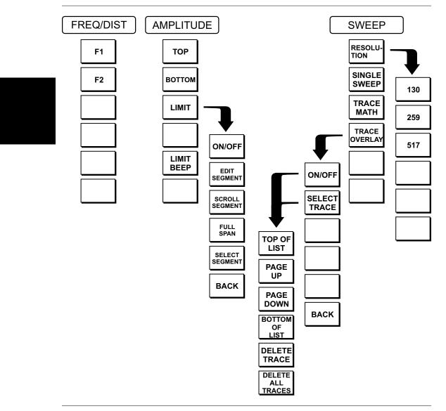
Figure 3-3. Frequency Mode Soft Key Labels
