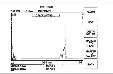
Figure 4-15. DTF - SWR Measurement Results (cable quality)
