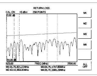
Figure 4-10. Cable SWR Measurement Results
