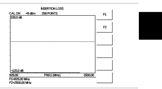
Figure 4-7. Insertion Gain Mode Calibration Results (RF Out connected to RF In)
