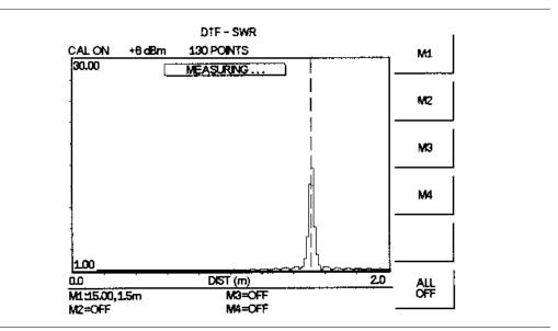
Figure 4-13. DTF - SWR Measurement Results (cable length)
