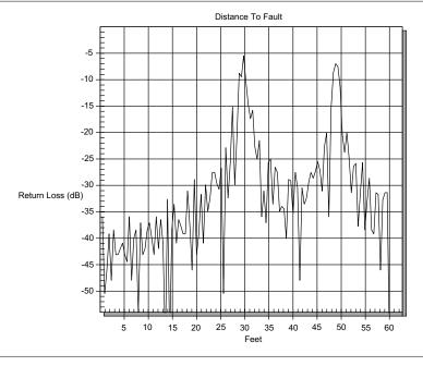
Figure 3-9. Rectangular Windowing Example
