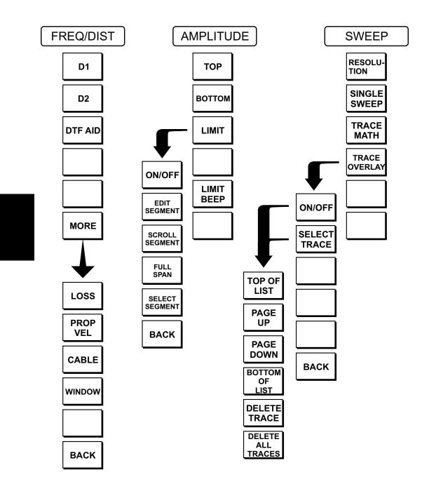
Figure 3-5. Distance to Fault Mode Soft Key Labels
