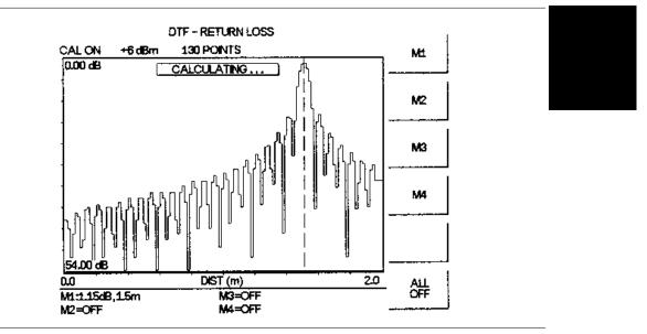
Figure 4-14. DTF - RETURN LOSS Measurement Results (cable length)
