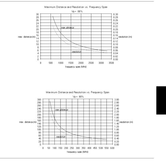
Figure 3-16. Maximum Distance and Resolution vs Frequency Span
