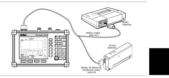
Figure 3-13. Site Master Printer Setup
