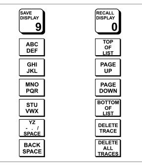
Figure 3-7. Save Display and Recall Display Soft Key Menus
