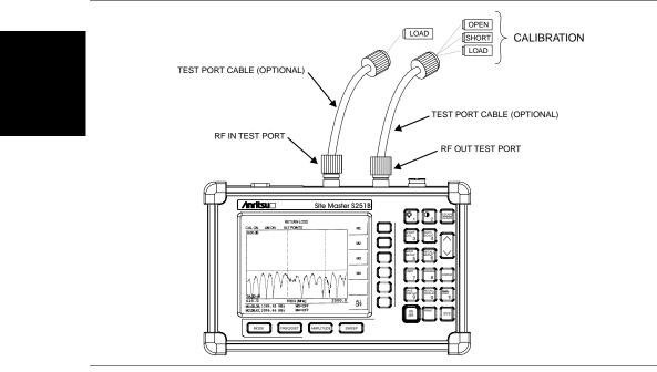
Figure 4-1. One-port Measurement Calibration Setup
