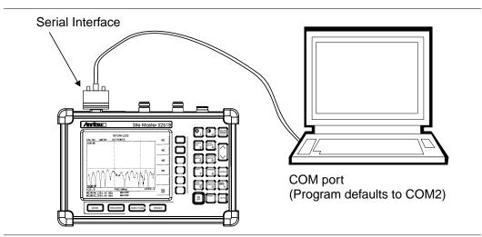
Figure 5-2. Serial Cable Connection
