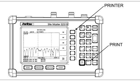
Figure 3-15. PRINTER Soft Key and PRINT Key
