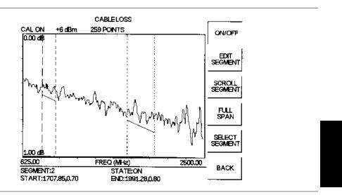
Figure 4-12. Cable Loss Measurement Results
