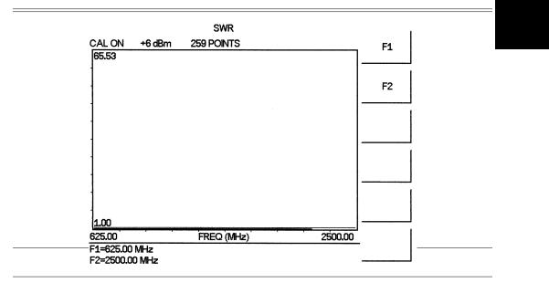
Figure 4-4. SWR Measurement Mode Calibration Results
