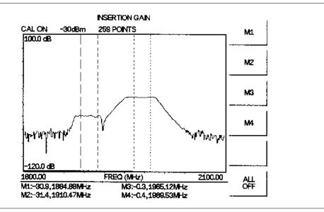
Figure 4-21. Measurement Display Showing Bypass Condition
