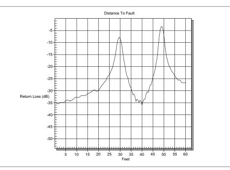
Figure 3-12. Minimum Side Lobe Windowing Example
