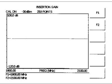
Figure 4-18. Two-Port Measurement Calibration Results
