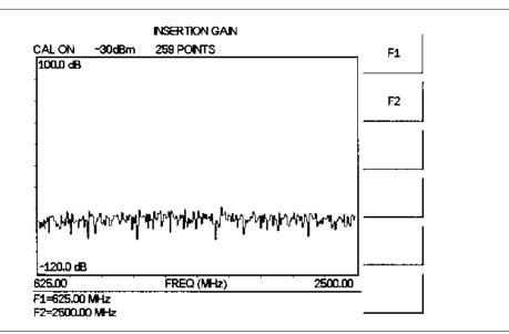
Figure 4-6. Insertion Loss Mode Calibration Results (Loads at RF Out and RF In)
