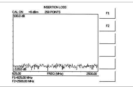
Figure 4-5. Insertion Loss Mode Calibration Results (Loads at RF Out and RF In)
