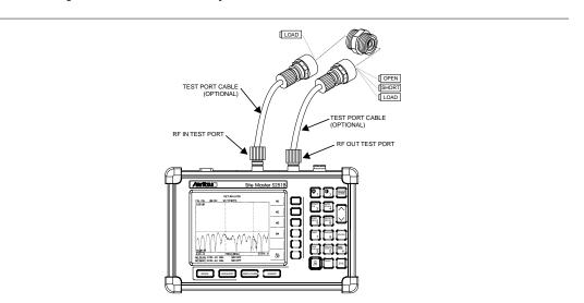
**Step 3.** Press the **ENTER** key to select the measurement mode.
