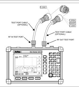
Figure 4-17. Two-Port Measurement Calibration Setup
