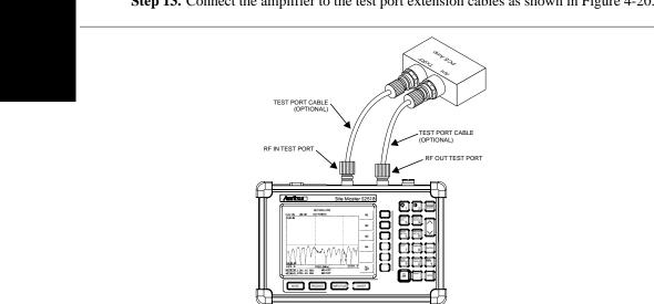
Step 13. Connect the amplifier to the test port extension cables as shown in Figure 4-20.
