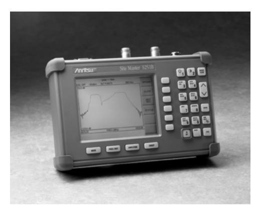
Hand-Held Tester for Transmission Lines and other RF Components
