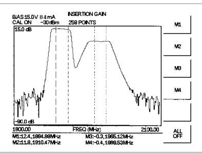
Figure 4-22. Measurement Display of Amplifier Gain
