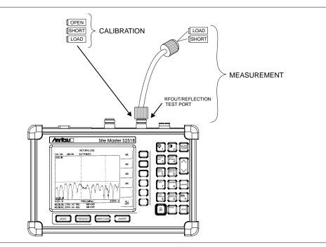
Figure 4-9. Cable Measurement Test Setup
