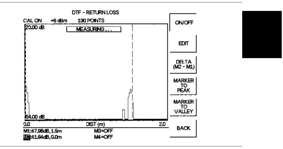
Figure 4-16. DTF - RETURN LOSS Measurement Results (cable quality)
